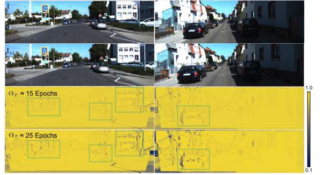
Fig. 3. \alpha_\tau over training time. \alpha_\tau varies spatially and over training time, and reduces weight of occlusions and disocclusions regions (e.g. the borders of the image and regions highlighted in green) as we become more confident in correspondences between I and I_{+1} .
