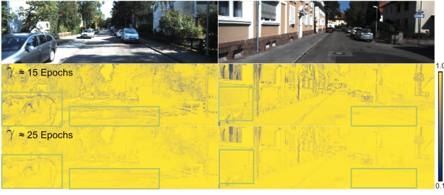
Fig. 4. \gamma over training time. \gamma is low during early stages of training and increases over time as mean residuals decrease. Regions of small residuals due to noise and slight illumination change (highlighted) are gradually regularized. For a local smoothness term, \gamma first allow the model to search for better correspondences and gradually impose smoothness.
